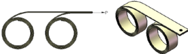
Tandem - this configuration does not add stability
